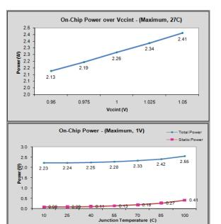
Figure 12: Power Consumption of Carry Skip Adder Using MTSG,PG and FRG Gates
