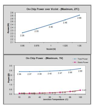
Figure 9: Power Consumption of Ripple Carry Adder using TSG Gates
