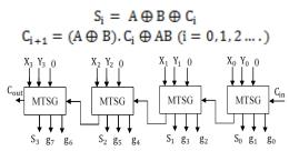
Figure 6: ripple carry adder using MTSG gates
