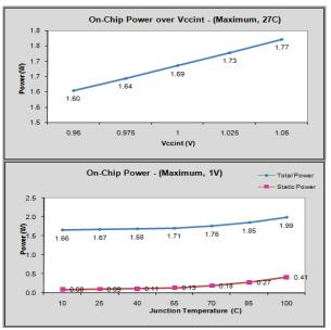
Figure 13: Power Consumption of Carry Skip Adder using MTSG,PG and MFRG Gates
