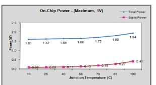
Figure 11: Power Consumption of Ripple Carry Adder using MHNG Gates
